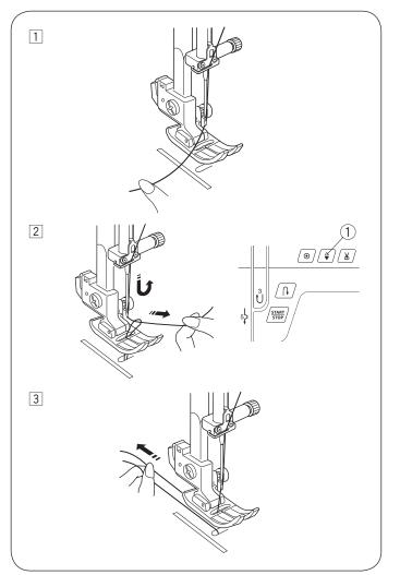
Drawing up the Bobbin Thread 1 Raise the presser foot. Hold the needle thread lightly with your left hand.
